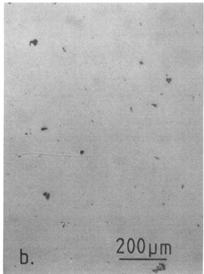
Fig. 18. Microstructures of hot-pressed materials: light micrographs of polished surfaces of materials prepared from (a) coated powder and (b) mechanically mixed powder.
